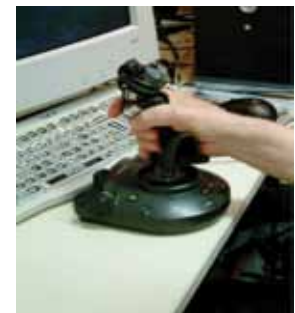
Computer joystick gives haptic feedback
