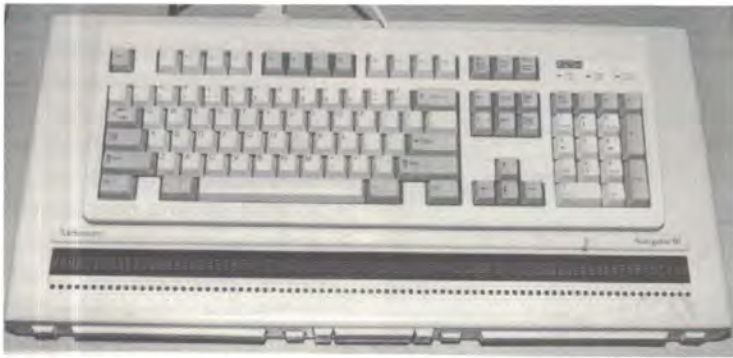
Keyboard with refreshable Braille
