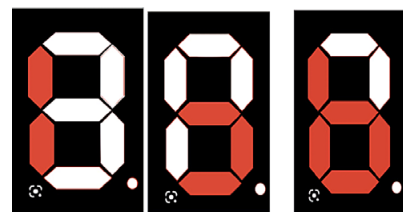
Fig 16. Composition of the letter “b” with the vertical line and the right loop displayed permanently on the 7-segment display
